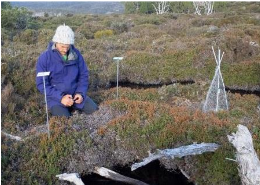
Figure 2: Example of a stainless tree guard (right) which we used for most of our caged interventions, and a typical open intervention (left). Poles are lengths of aluminium tubing, pushed or hammered into the ground. Mesh on the tree guard is stainless steel chicken wire.
